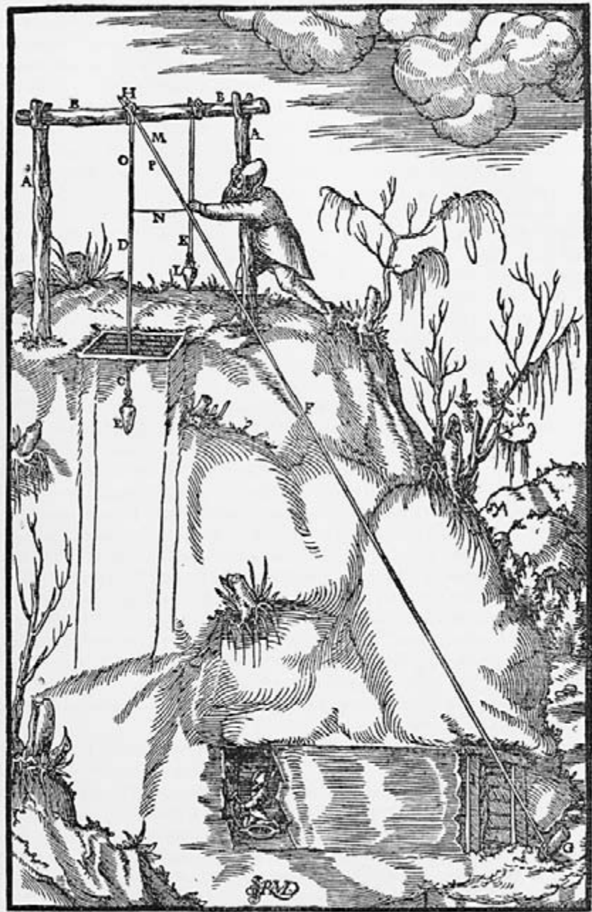
Figure 1.5. A surveyor depicted in the mining book De Re Metallica , first published in 1556. Such surveyors measured triangles and reproduced their results in full scale on the ground in an open-air “surveyor’s field.” From Georgius Agricola, De Re Metallica , translated by Herbert Clark Hoover and Lou Henry Hoover (London: Mining Magazine, 1912), 131.
