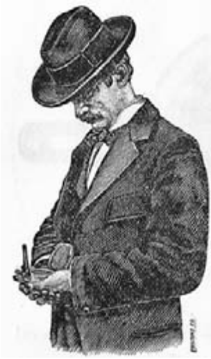
Figure 3.1. David W. Brunton's innovative pocket transit dispensed with a tripod by instead requiring the user to hold it tightly against his midsection with both hands, craning his neck downward to peer into the device. Here, it is being used to measure a course or horizontal angle. When held properly, the sight-lines worked and the user received usable results. The lack of a tripod made using the pocket transit an easy way to achieve fast results with rough accuracy, and this was key to collecting the extensive geological information at the heart of the Anaconda System of mapping. From Dunbar D. Scott and others, The Evolution of Mine-Surveying Instruments (New York: American Institute of Mining Engineers, 1902), 90.
