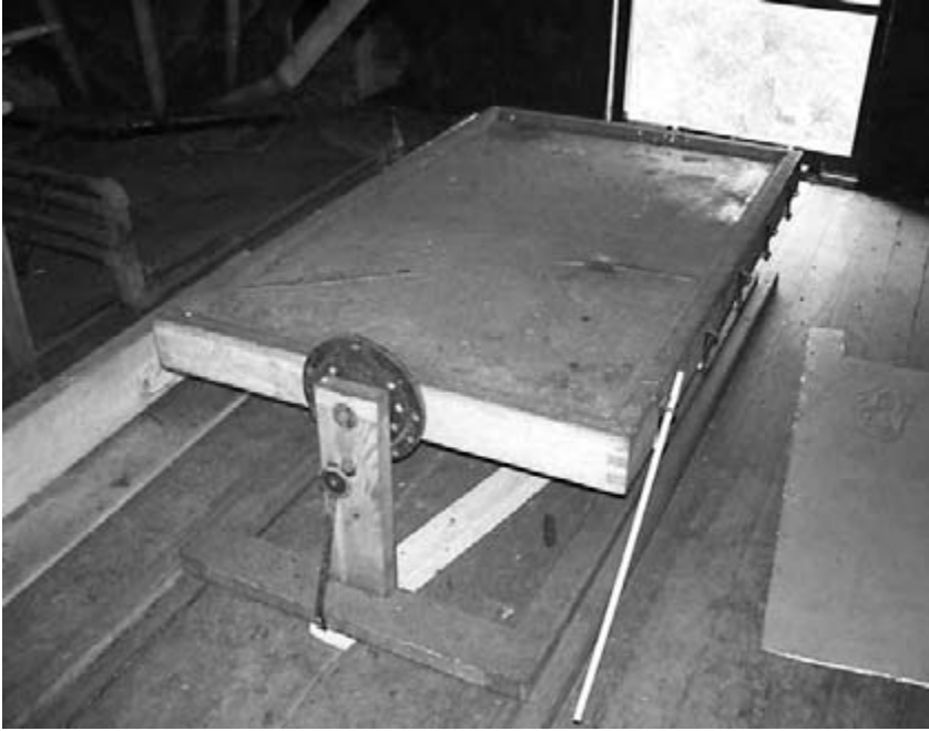
Figure 1.3. A drawing on semitransparent tracing linen would be placed along with sensitized blueprint paper in this solar-powered blueprint frame, and the assembly would be left in the sun to expose the print. This example, likely circa 1890s and located in situ in the attic of the Quincy Mining Company office building, was pushed out the attic window on rails. Quincy Mine Office building, Keweenaw National Historical Park, Hancock MI. Photo by Eric Nystrom, 2010.
