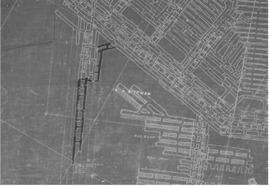
Figure 1.1. The 1964 map of the Saxman Mine, found in a local historical society, depicted tunnels not shown on earlier maps. These excavations, jutting down from the main workings in center-left, filled with water and flooded the neighboring Quecreek Mine when miners inadvertently broke through. Document 39230403, Office of Surface Mining, Reclamation and Enforcement's National Mine Map Repository, Pittsburgh, PA.
